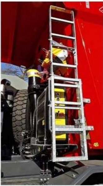
Figure 2. The new generation of the HYVA ALPHA hydraulic cylinder provides shorter body lifting and lowering time.
