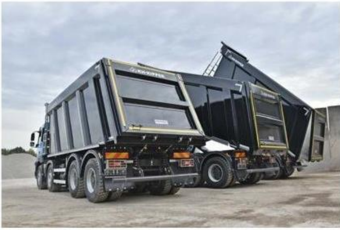
Figure 1. KH-KIPPER W1C mining body for coal transport.
