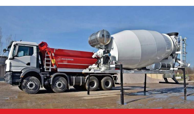
The exchangeable system is a special construction designed for exchanging different types of bodies on truck chassis. It is a complete solution for concrete plants, mines as well as gravel pits and it improves the vehicle's functionality all year round.
